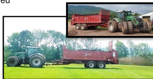
Albanos Precision Application Variable-rate semi-solid manure spreader
