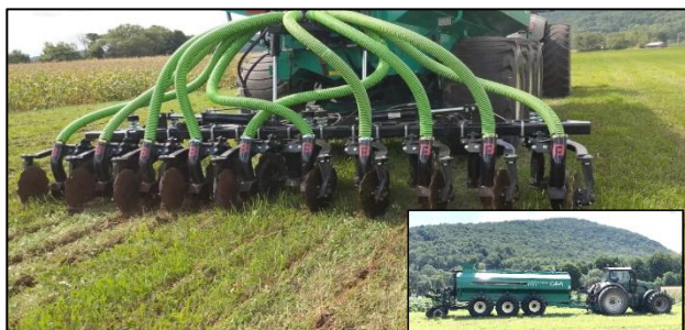
Variable rate disc-coulter liquid manure injection tanker tool bar
